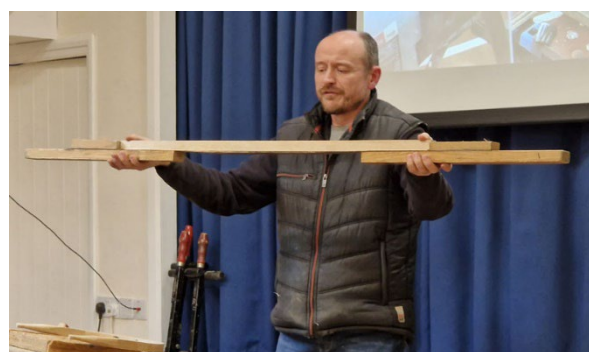
The steamed straight oak timber fits along the strap and meets the chocks at each end for perfect placement
