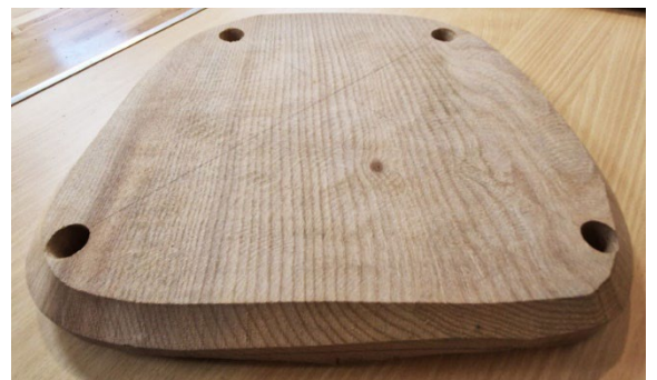
Drilled seat with further shaping applied, requires sanding and further finishing
