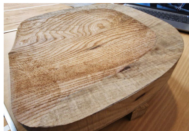
The Arbortec shaped seat without any finishing
